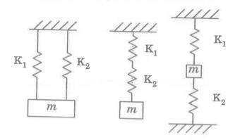
13. What is the value of C such that the system in critically damped if m = 20 kg and K = 10,000 N/m?
