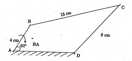
13. Synthesis a four-bar Crank-Rocker Quick return mechanism with following data:
