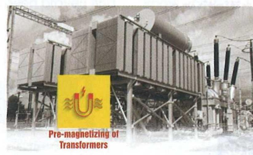
Transformer is energized by closing circuit breaker, with system voltage being applied on transformer instantly. This switching introduces an asymmetrical magnetic flux in core, driving the transformer into saturation. As a result, high magnetizing current is produced in the winding. Magnitude of this current may reach upto 10 times of the rated current.
