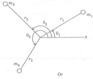
12. The connecting rod of a three-cylinder air compressor are coupled to a single crank and the axis are at 120° to one another. Each connecting rod is 180 mm long and the stroke is 120 mm. The reciprocating parts have a mass of 1.8 kg per cylinder. Find the magnitude of the primary and secondary forces. When the engine runs at 1200 r.p.m.
