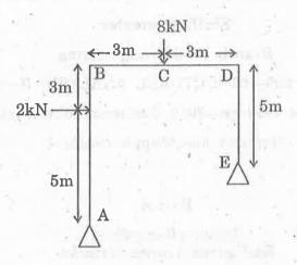
13. Analyze a frame shown below using cantilever method. Draw the BMD.
