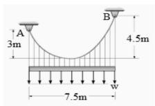
8 a) A three-hinged parabolic arch is loaded as shown in figure. Calculate the location and magnitude of maximum bending moment in the arch. Draw bending moment diagram.
