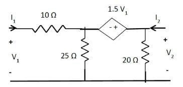
b) Two identical sections of a network shown in the figure are connected in series. obtain the Z parameters of the combination and verify by direct calculation (8)
