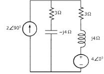
c) Find the value of  $V_0$  such that no current flows through  $4\Omega$  resistor.
