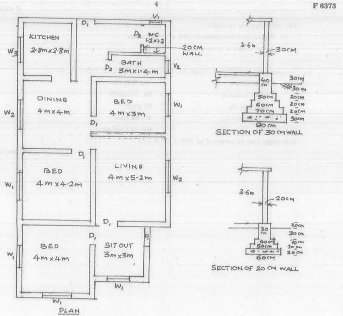
DOORS D1 = 1.2m x2.1m D2 = 1 m x 2:1m WINDOWS W1 = 1.5m x 1.35m Wa = 2 m x 1.35 m W3 = 1.5mx0.75m VENTILLATOR
