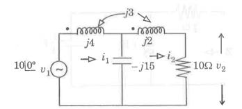
15. Determine the circuit constants in the circuit shown if the applied voltage is  $v(t) = 100 \sin (50t + 20^{\circ})$ . The true power in the circuit is 200 w and pf is  $0.7 \circ 7$  lagging.
