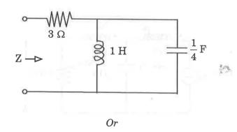
18. For the network shown determine the Transfer function  $G_{21}(s)$  and Transfer Impedance  $Z_{21}(s)$ and driving point admittance  $Y_{11}$  (s).
