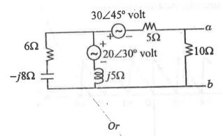
14. Draw the graph of the network shown in the figure below. Write the cut-set schedule and calculate all branch voltages and branch currents.
