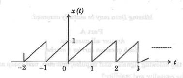
(b) Find the real and imaginery parts of the Fourier Transform of the pulse x(t) shown in figure.
