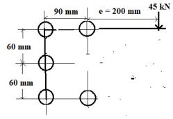
The shear stress is 110 MPa and the crushing strength is 150 MPa. Find the diameter of the rivet.
