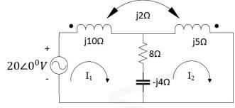
b) If the network given below is connected across a 230V, 50Hz AC source, (7) determine the current supplied by the source.
