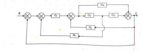
2 a) A positional control system with velocity feedback is shown. What is the response c(t) to (8) unit step input? Given that  $\varepsilon = 0.5$ . Calculate rise time, peak time and settling time.
