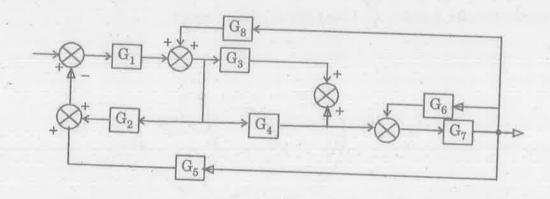
14. Draw the Signal flow graph and determine the overall Transfer function:
