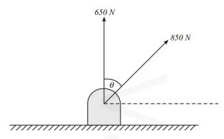
11 b Four forces are acting on a bolt as shown in Figure 3.10. Determine the magnitude (7) and direction of the resultant force
