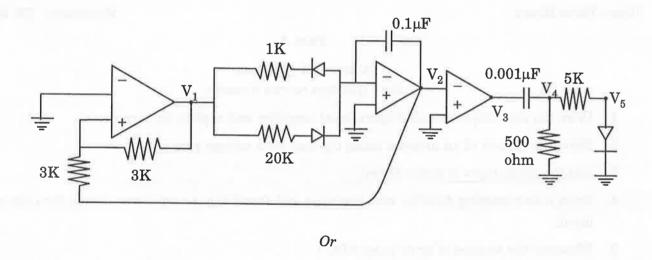
14. Cascade an active LPF and BPF to design a wide band pass filter which passes frequencies from 20 Hz to 2 kHz using Op-amp.
